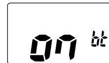
Battery voltage indication ON
